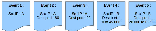
Fig. 1. Event 1, Event 2 and Event 3 report different traffics from the same host. A same port scan is reported by two events; Event 4 identifies only a part of it (beginning of the port range), whereas Event 5 identifies another part (the end of the port range).
