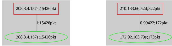
(a) Both methods detect the same host infected by the Sasser worm. (b) The gamma-based method reports the destination of anomalous traffic whereas the Hough-based one reports the source of it.
